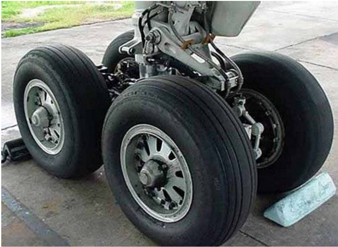
Boeing 757 main landing gear wheels
