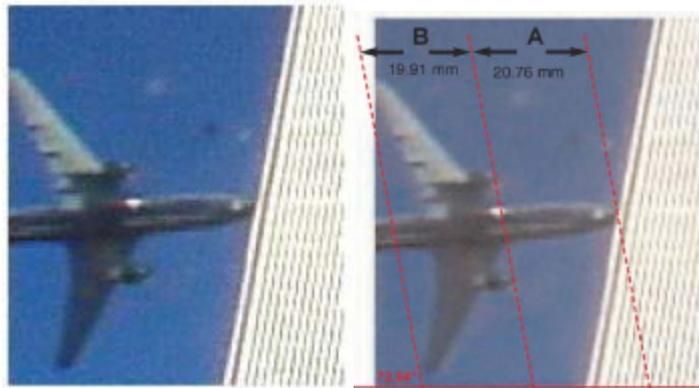
A line is drawn connecting the trailing edge of the wingtips, and another connecting the fronts of the engine nacelles. Distances are measured from the nose tip to the engine fronts, from the engine fronts to the wingtips, and comparisons are made to known measurements of the 767-200 and 767-300.
